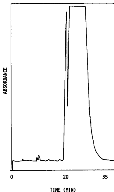
Fig. 3. Injection of 25 mg of 1a-1b test mixture. Column, Whatman Partisil 10 silica Magnum 9 (50 cm \times 9.4 mm I.D.); mobile phase, dichloromethane-methyl tert. -butyl ether (93:7) at 4.0 ml/min.
